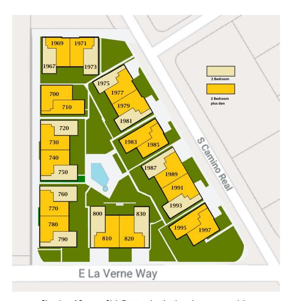
Site plan of Country Club Estates showing how Jones arranged the different structures/units. Note how the architect positioned the end units to create wall space for patios.
